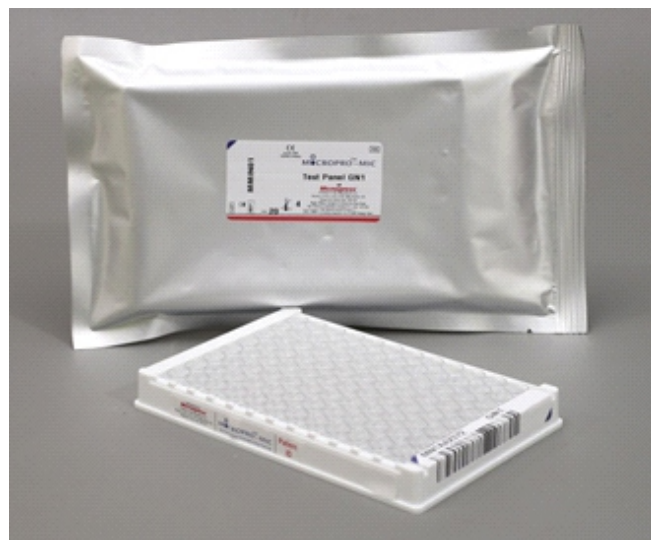
Fig no. 1: 96-well microtitration plate used for Microdilution (Micropro™-MIC)
