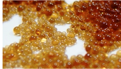
Resin beads used in ion exchange water treatment.
