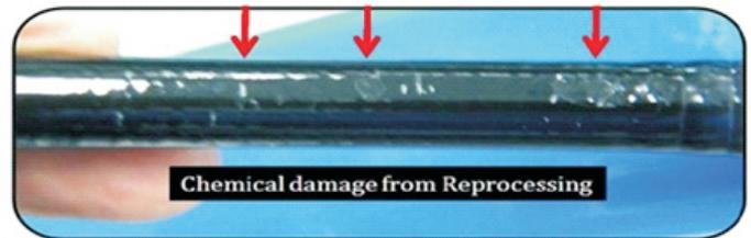
Figure 3. Chemical Damage from Reprocessing
