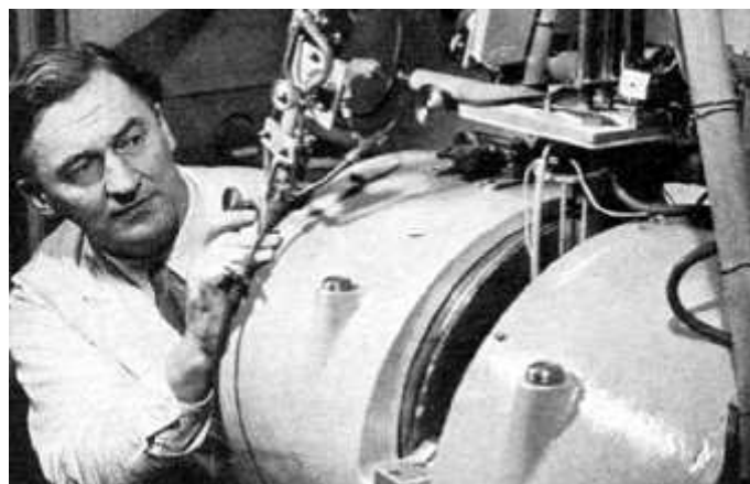
Nobel Laureate Hugo Theorell with the "home-made" magnetic weighing machine that was constructed at Karolinska Institutet.
